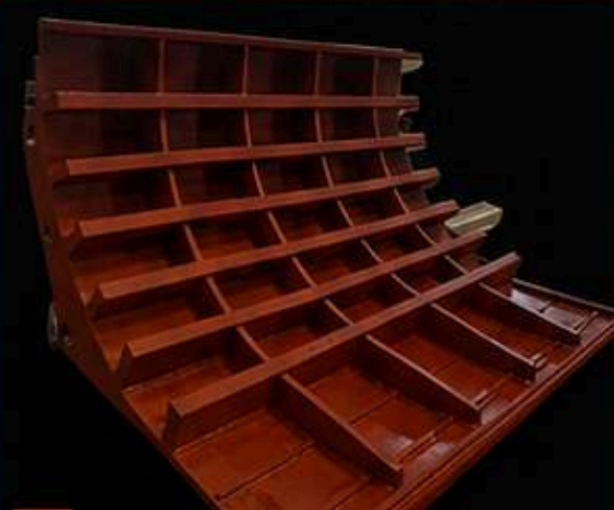
FIBRIZER/SHREDDER ANVIL PLATE
